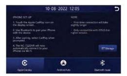
Before connection, press the "BT Manage" button if you wish to change the Bluetooth name and settings. NC-722DVR\_XXXX (where XXXX is the unique code) is the default Bluetooth name.
